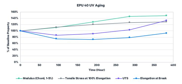
ASTM D4459: Q-Sun XE-1, 0.8 W/m² at 420 nm, 55  $^{\circ}$ C ASTM D412: Die C, 500 mm/min, average values represented
